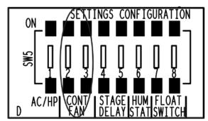
air handling unit can produce, not the maximum CFM set on the HI COOL setting. For example, a C36D air handling unit maximum CFM is 1350 CFM. Regardless of HI COOL setting, a continuous fan address of 11 will result in 1350 CFM during a continuous fan call. A continuous fan call
