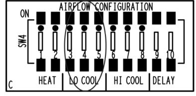
350 - 400 CFM per ton and low-speed airflow is approximately 67% of high-speed airflow. To locate the correct address, reference the airflow data table in the air handling unit installation manual.
