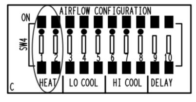
If a multi-stage outdoor unit is utilized, a LO COOL address must be set for required low-speed airflow. This address is for both heat pump heating and air conditioning compressor airflow speed which will occur
