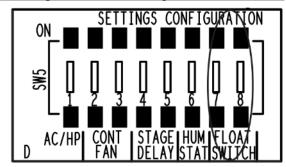
settings menu, the FLOAT SWITCH setting must be changed from its default (disabled) setting. If using a normally closed switch, choose Enabled (Open). If using a normally open switch, choose Enabled (Closed).
