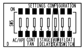
The variable speed air handling unit control can monitor an accessory float switch connected to the float switch input on the control. The feature is only available when using a communicating room thermostat.
