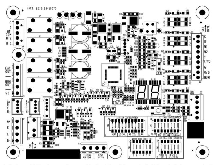
In the lower right-hand corner, there are 4 banks of dipswitches each of which are in their own quadrant labeled A, B, C, or D. Each bank of switches is labeled SW2, SW3, SW4, or SW5. Each switch has an ON or OFF position. Every individual switch comes from the factory in its OFF position.
