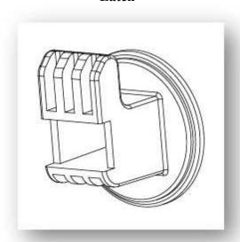
The new handle/latch is designed to eliminate the failure modes of the current knob and will be compatible with all applications where the 1/4 turn knob is used.
