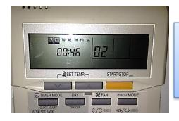
After installing the switch the next step is programming. You must program the unit for "Forced Stop". Function 46 setting value 02. This can be found in the installation manual for the unit. Once programming is finished power must be reset for 5 minutes.
