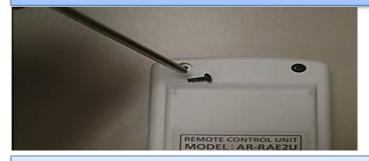
Remove all screws from behind the remote control and open up.
