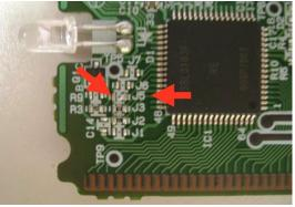
To make the conversion, remove the number 5 jumper from the remote's circuit board.
