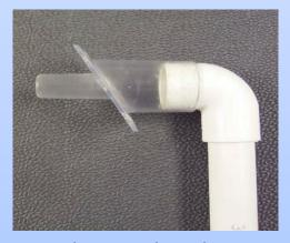
Make sure the adaptor fits into the drain port, after sanding down both components.
