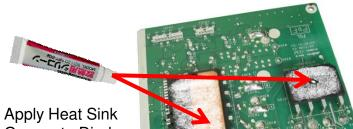
Grease to Diode Bridge and IPM IC
