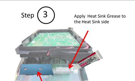
Place insulation sheet on the heat sink , Diode Bridge Side (Blue)
