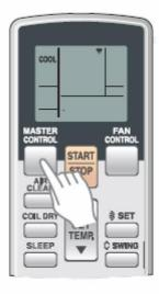
Press the MASTER CONTROL button to exit the programming mode.
