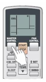
Press the MASTER CONTROL button for 5 seconds or more until a, b, c, or d displays.
