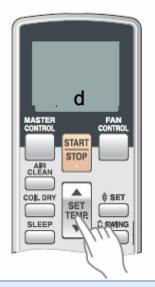
Press the SET TEMP button to select the desired code. (a,b,c,d)
