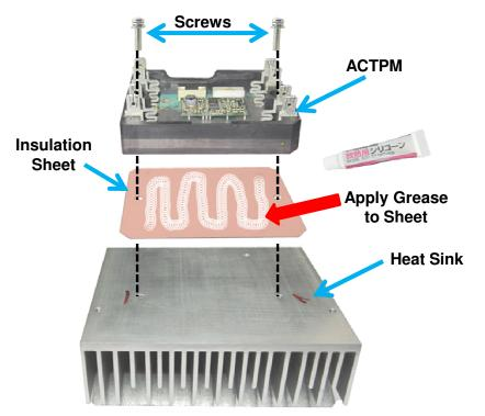
ACTPM, IPM, INVERTER CONTROL PCB and DIODE BRIDGE must have the grease spread on and fastened to the heat sink with the enclosed screws.
