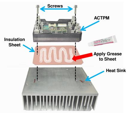
ACTPM, IPM, INVERTER CONTROL PCB and DIODE BRIDGE must have the grease spread on and fastened to the heat sink with the enclosed screws.
