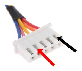
If you read open or shorted on any of the wires or out of the range listed, replace the stepper motor.
