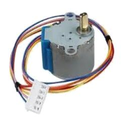
To complete this test shut off main power, Unplug stepper motor from board and place your meter in Ohms  $\Omega$ . Place Your Black (-) lead on the Red wire and your Red (+) lead to each wire and you should read the same values on all wires.
