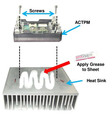
ACTPM, IPM, INVERTER CONTROL PCB and DIODE BRIDGE must have the grease spread on and fastened to the heat sink with the enclosed screws.
