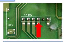
On multi-zone systems look for CN802( fan motor) Use pin 3 for DC ground.
