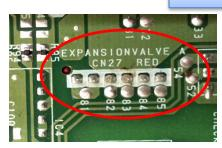
Test on all 6 solder points on the board and verify voltage reads 12-13
