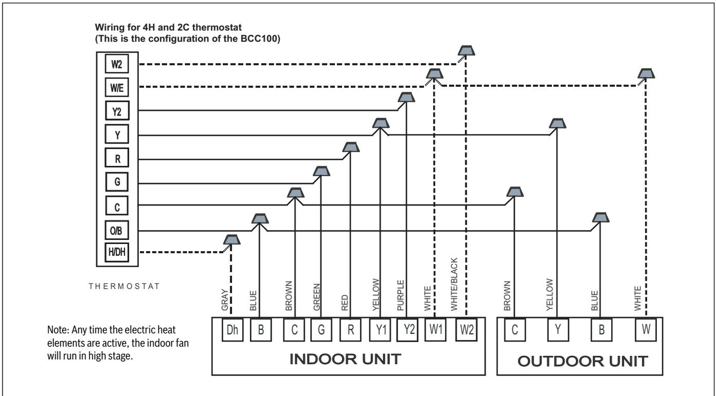
Figure 29 Thermostat Wiring Diagram for BOVB20/BVA20 Matched System
