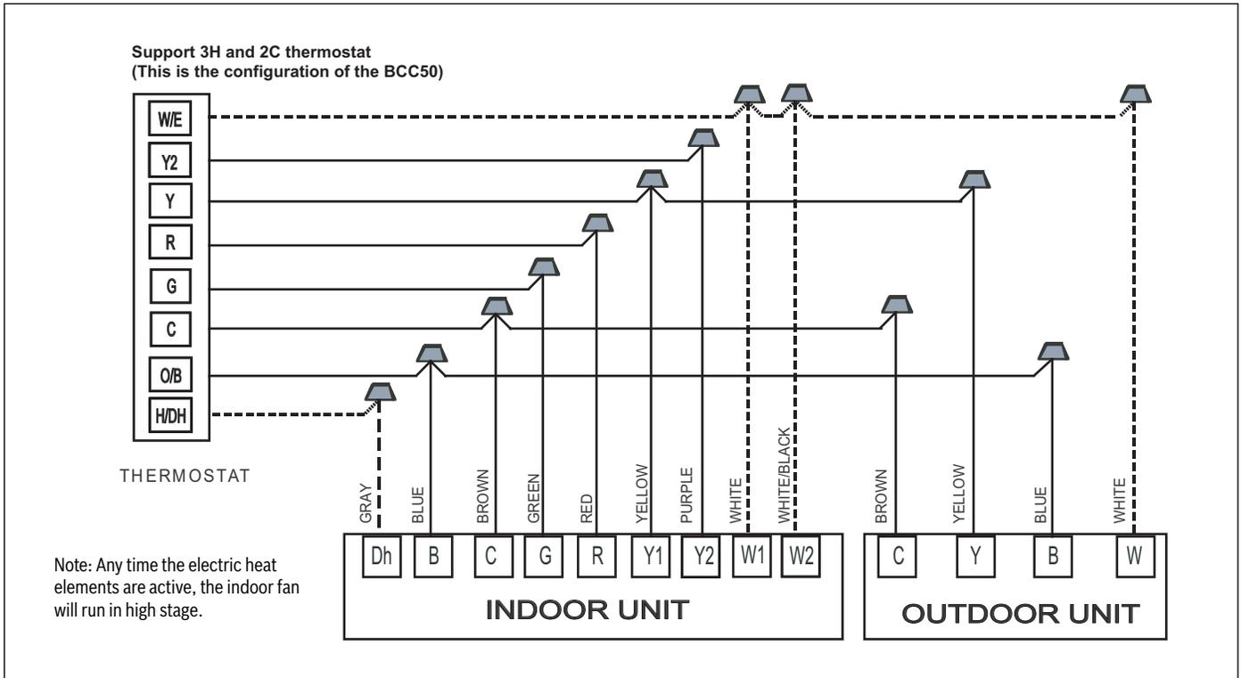
Figure 28 Thermostat Wiring Diagram for BOVB20/BVA20 Matched System
