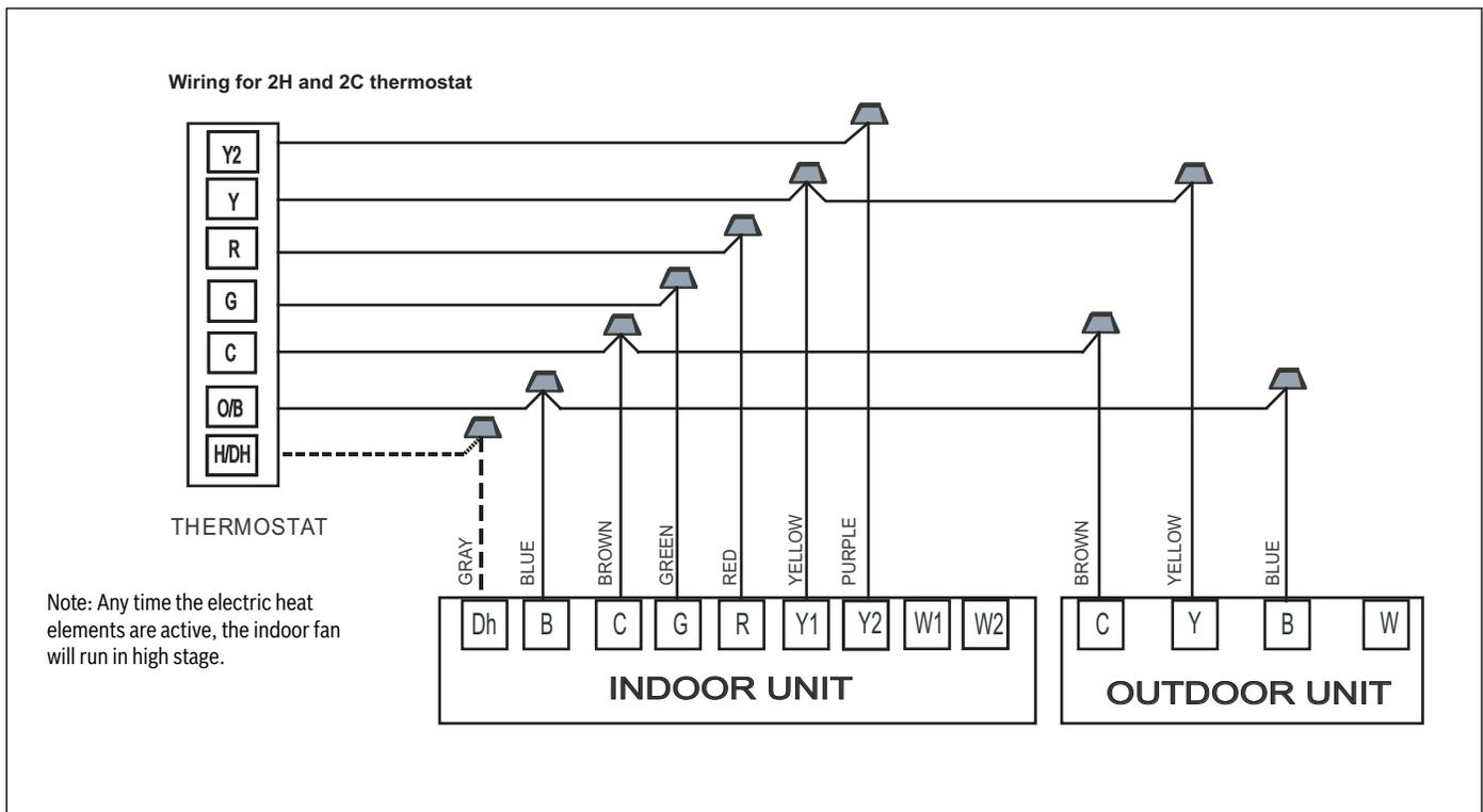
Figure 31 Thermostat Wiring Diagram for BOVB20/BVA20 Matched System
