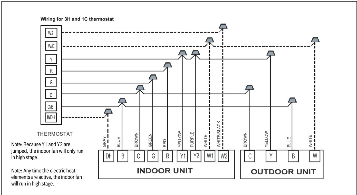
Figure 30 Thermostat Wiring Diagram for BOVB20/BVA20 Matched System
