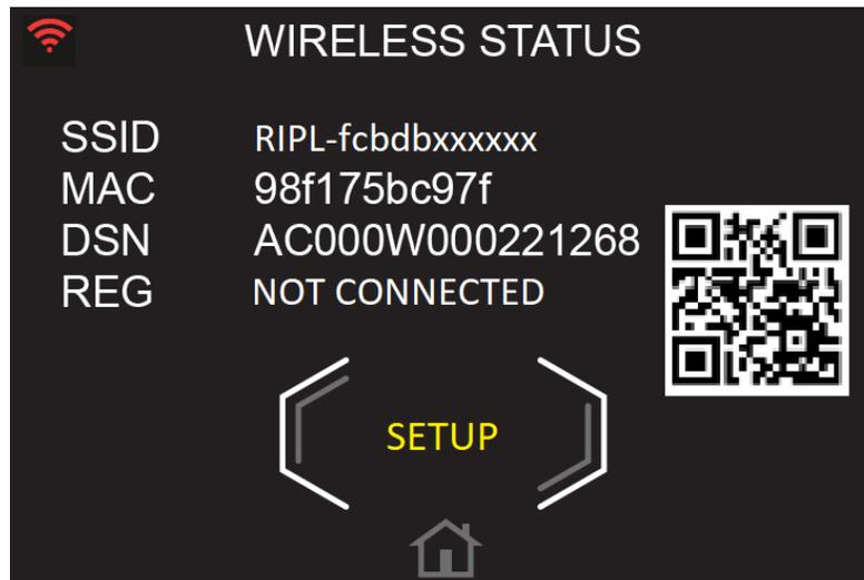
As previously mentioned if the thermostat does not have the latest version of software installed on it, the QR code will not be present. The mobile application has a selection to enter the code manually. The code is the thermostat SSID which begins with RIPL- and is case sensitive. An image of manual entry is shown below.
