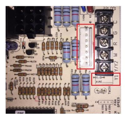
Note the red rectangle outline with the wire jumper inside it. It is labeled Y1. This is correct for the single stage PSC model control board.
