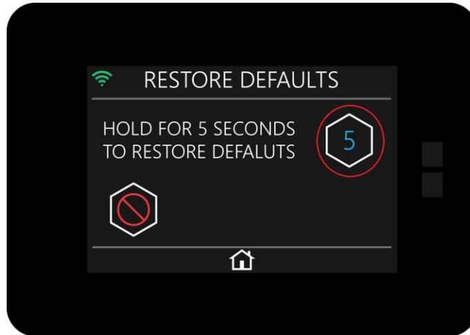
After factory defaults have been restored, the thermostat will find the previously wired communicating equipment and it will enter the auto setup mode.
