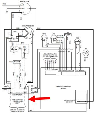
Implemented in August 2018, only the generation 2 YHE and RHP14L models were built with a true ECM motor, module, and wiring. Below is a wiring schematic showing where the ECM module's low voltage black wire is to be connected to the contactor 24 VAC coil.
