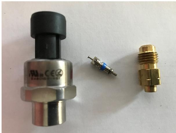
To install a flare type transducer in place of a sweat type transducer, the sweat type transducer must be removed and replaced with a brass ¼ male flare connector like the one shown above. Since this is a brass to copper braze connection, a technician very proficient in brazing must make the repair.
